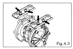
• Turn over the main body assembly. [Fig.4.3] Remove the 4 retainer bolts from the in manifold, and remove the in manifold. [Fig.4.3]
