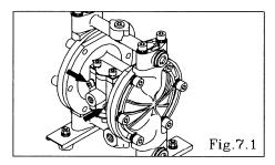
• Remove the 2 retainer from the spool valve case, and remove the spool valve case. [Fig.7.1]
