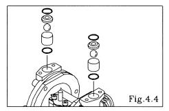
• Remove the O ring, valve seat, ball and valve stopper. [Fig.4.4]
