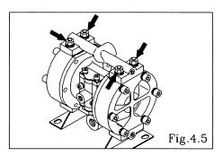
• Remove the 4 retainer nuts from the out manifold, and remove the out manifold. [Fig.4.5]
