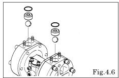
Remove the O ring, valve stopper, ball and valve seat. [Fig.4.6]
