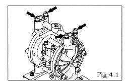
• Remove the 4 retainer bolts from the out manifold, and remove the out manifold. [Fig.4.1]
