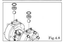
• Remove the O ring (excluded BPC, BPN), ball and valve seat. [Fig.4.8]
