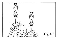
• Remove the O ring, valve stopper, ball and valve seat. [Fig.4.2]
