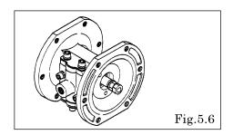
• Remove the center disk and diaphragm from the opposite side using the double nut. [Fig.5.6] Be careful not to scratch or score the center rod.
